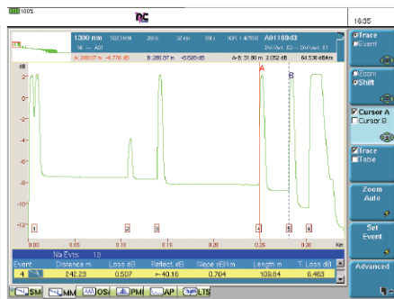
An example of a ghost on the OTDR trace
