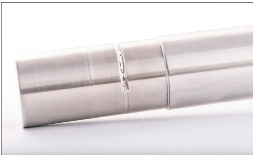
Figure 2. PAT-L showing transmission measurement gap
